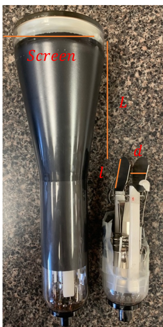
Fig. 8 Inside of broken CRT and working CRT
